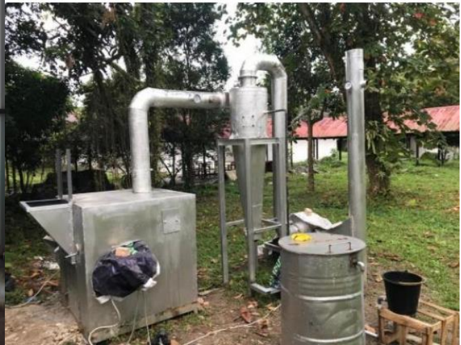
1a. The incinerator as a result of Dr. Eng Hafizhul Khair et al to process domestic waste
