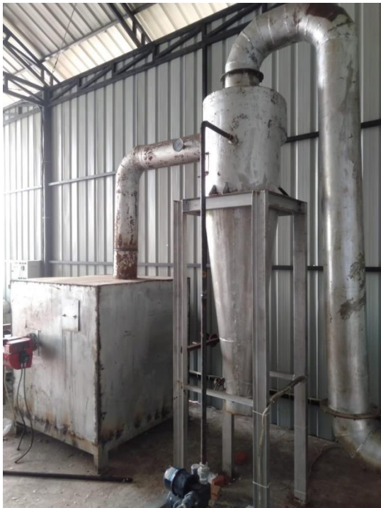
1a. The incinerator as a result of Dr. Eng Hafizhul Khair et al to process domestic waste
