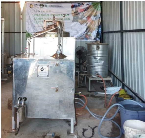
1b. Pyrolysis equipment which is a grant from Earthwise Consulting Japan to process plastic waste into fuel oil
