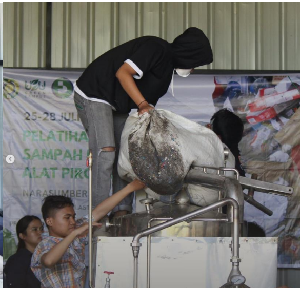
1b. Pyrolysis equipment which is a grant from Earthwise Consulting Japan to process plastic waste into fuel oil
